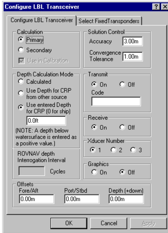
See the LBL ACOUSTICS chapter for details on setting these parameters. They are the same across all LBL TRANCEIVERS except for the **Transmit Code**. The “transmit code” must match exactly what was entered as the receive value or code for the fixed transponders. Example: 9.0 is not the same as 9.00.
